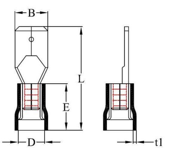
Male Insulated Terminal (Yellow)with anti-vibration insert Size: 6.4 x 0.8mm **B** Tab size: 6.30mm **L** Length: 24.5mm **D** Diameter: 4.90mm **E** Insulation Height: 13.5mm **t1** : 0.8
